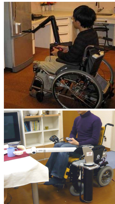
Fig. 6: Robotic arms for persons with disabilities in upper-limb (top: iARM, bottom: RAPUDA)
